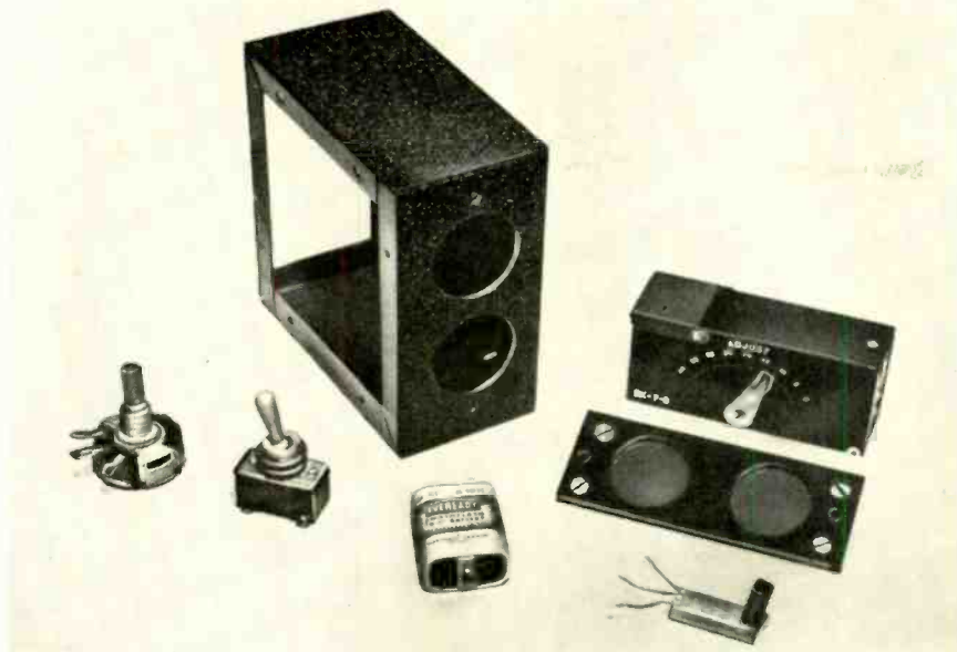
Photo of all parts used in the relay. The transistor, used in other experiments, is cemented to a small plastic block which supports its fragile leads.
